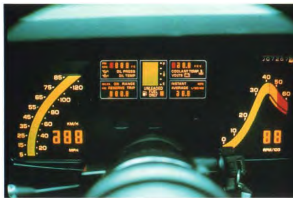
Plate 11. Automobile dashboard with liquid crystal display. (Courtesy of General Motors Corporation)
