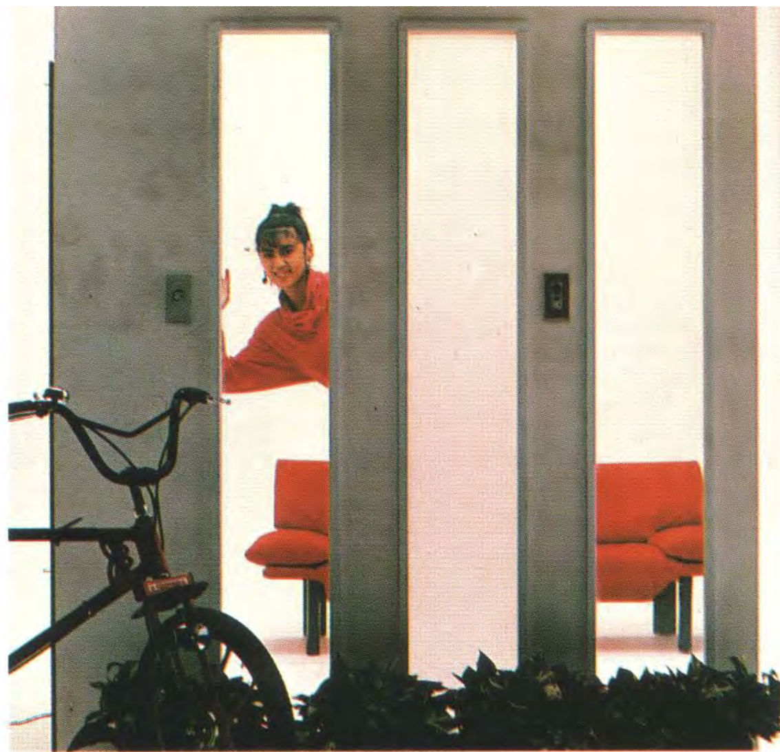
Plate 9. Switchable light panels. The middle panel is in the opaque state, while the two outside panels are in the clear state. (Courtesy of Taliq Corporation)
