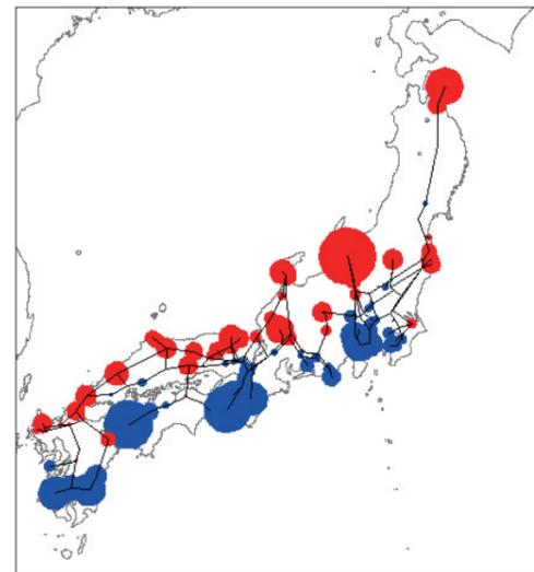
Figure 2. The distribution of the estimated risk against GICs for a 500-kV transmission network in Japan. The magnitude of the GIC flowing at a substation is indicated by the radius of the circle
