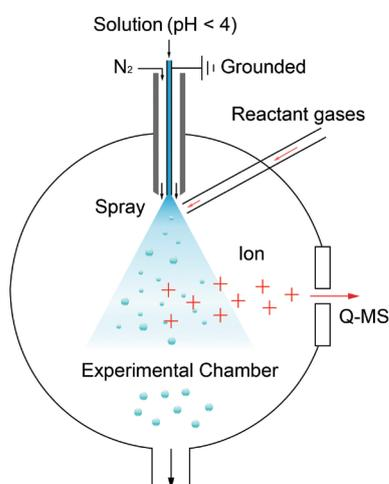
Figure 2: A scheme illustrating online detection of reaction intermediates forming at the air–water interface of microjets. The microjets are exposed to reactant gases, and the ionic products re-emitted into the gas phase are detected by quadrupole mass spectrometry (Q-MS).
