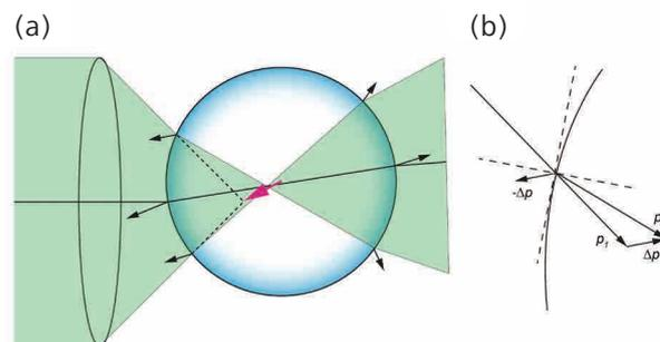
Figure 3: A schematic illustrating optical trapping of single aerosol by focusing laser light. (a) Optical forces dragging the particle to the focus center arises from (b) refractions at interfaces.
